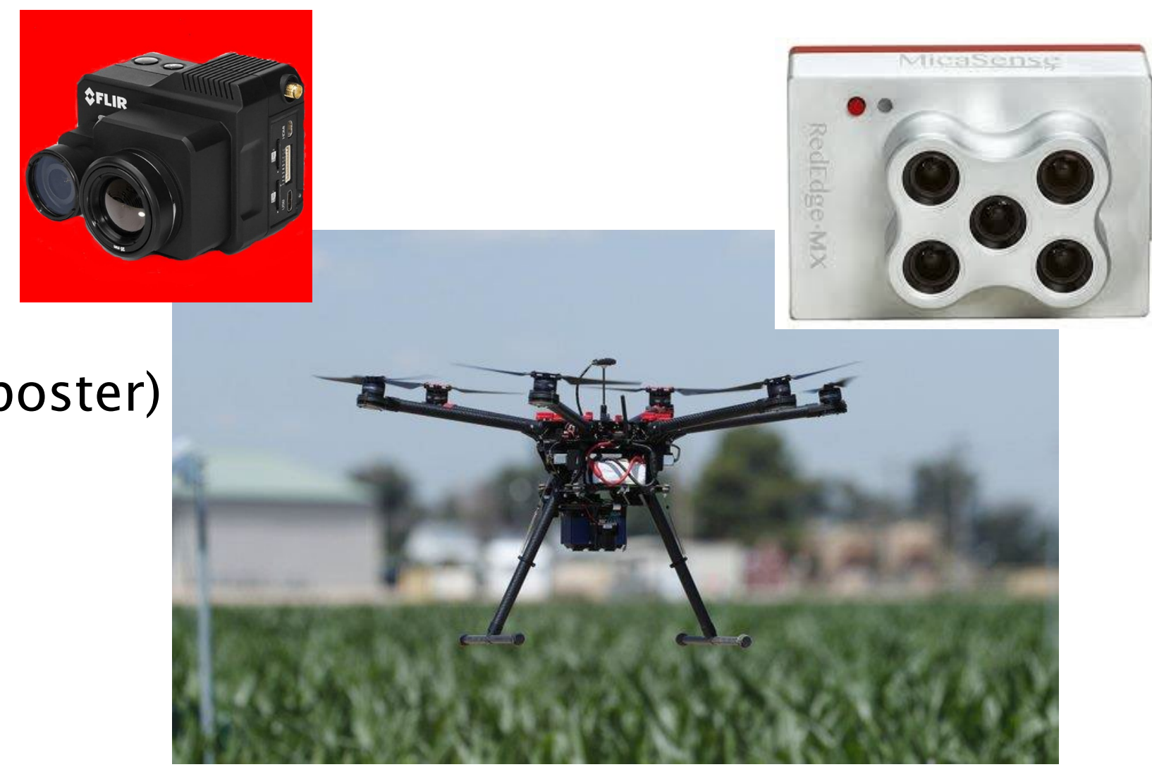
Fig. 4. UAV system with an RGB, thermal, and multispectral camera.
