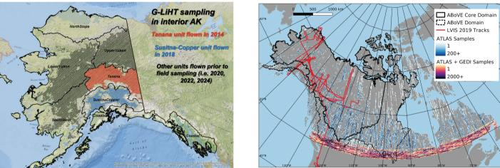
Left: Goddard's Lidar, Hyperspectral, and Thermal Imager (G-LiHT) flight lines in Alaska. Right: Airborne lidar (LVIS) in red lines, satellite lidar (ICESat-2 ATLAS & GEDI) in points, indicating sample density, across study domain.
