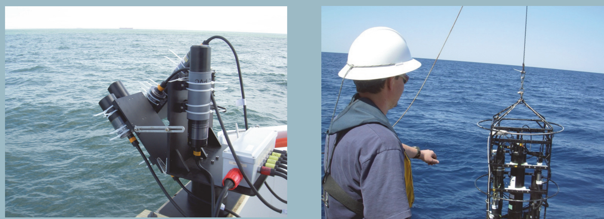
Figure 2. HyperSAS hyperspectral radiometry system (Satlantic, Inc.) deployed aboard the R/V Cape Hatteras in April 2009. In addition to radiometry measurements, discrete profiles of spectral absorption and backscattering were determined using a WETLabs, Inc. (now Seabird, Inc.) ac-9 absorption/attenuation meter and ECO-BB9 and ECO-VSF3 backscattering meters . Discrete water sample analysis included HPLC phytoplankton pigments, total suspended particulate matter, and total particulate carbon .
