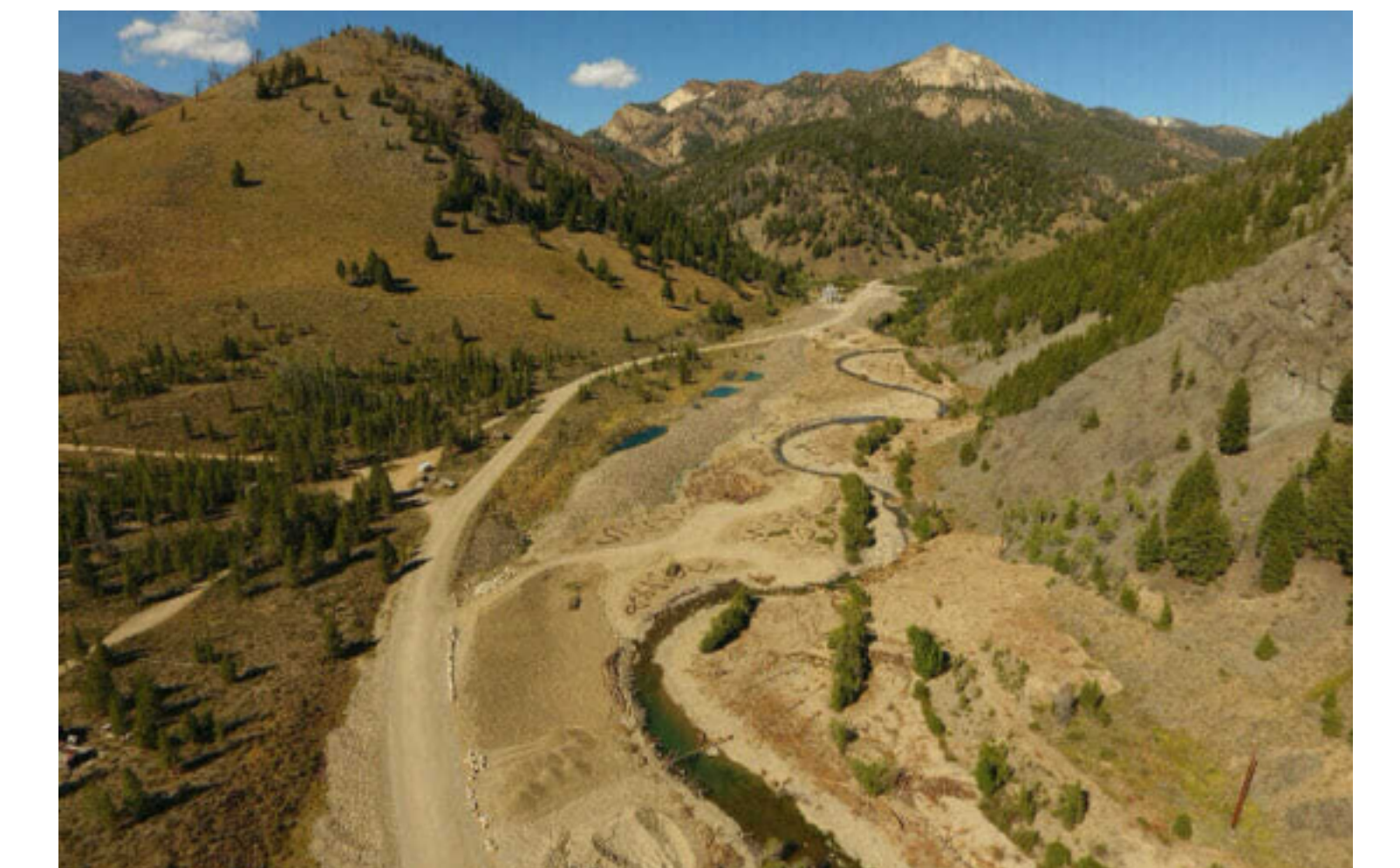
Yankee Fork of the Salmon River restoration project led by Trout Unlimited. Beginning in 2012, this project sought to increase channel complexity, riparian vegetation, and fish habitat. Beavers established in 2015 and continued the work.
