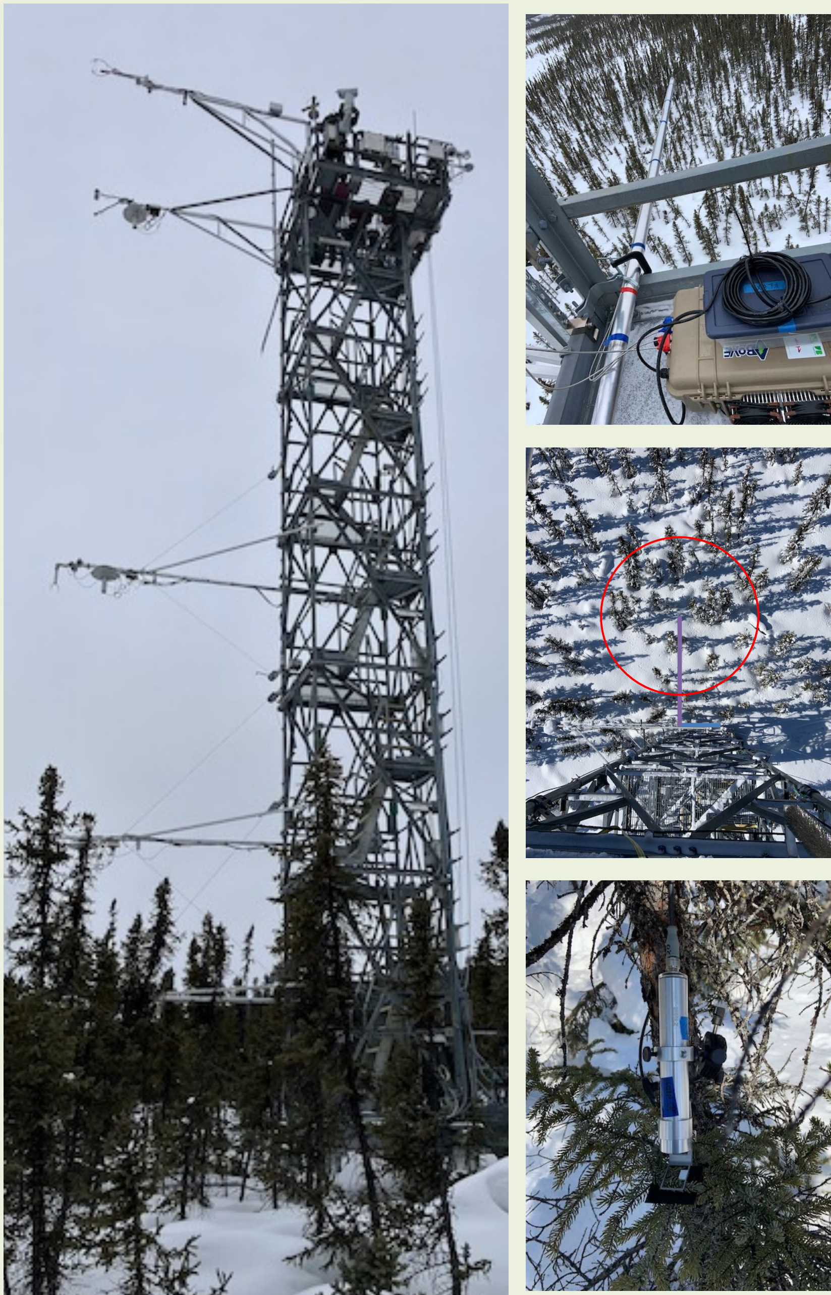
Left: Caribou Creek NEON flux tower, Right top: FLoX mounted on top of tower, Right middle: Field of view of FLoX shown by red circle, Right bottom: a MoniPAM sensor head attached to spruce branch
