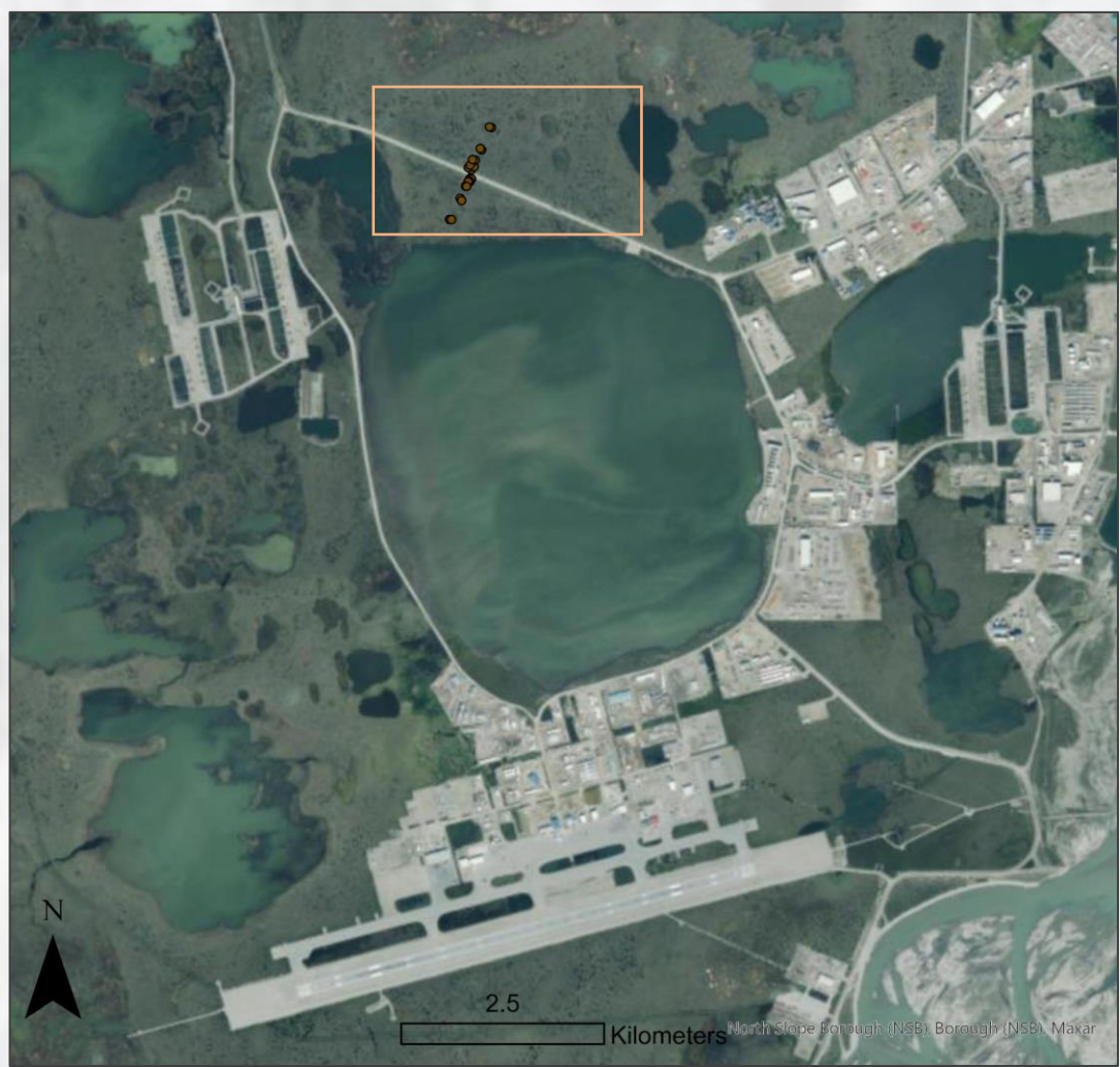
Figure 6: Study area (orange box) located north of the Prudhoe Bay airport. Ground temperature data used (locations shown as points in figures 6, 8 and 9) provided by Walker et al., (2015 and 2016). Measurements taken at 5 m from the road were omitted from analysis. Measurements included were 10 m, 25 m, 50 m, 100 m and 200 m from the road. Image is an ESRI World Imagery basemap image (7/15/2019) accessed using ArcGIS Pro v.2.7.
